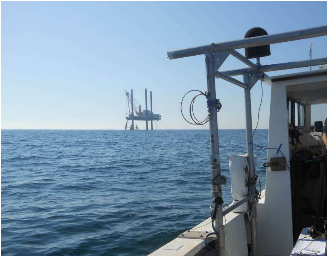
Figure 2-2 McMaster deck showing microphone positioning and high performance windscreen (jack-up barge for piling in background)
