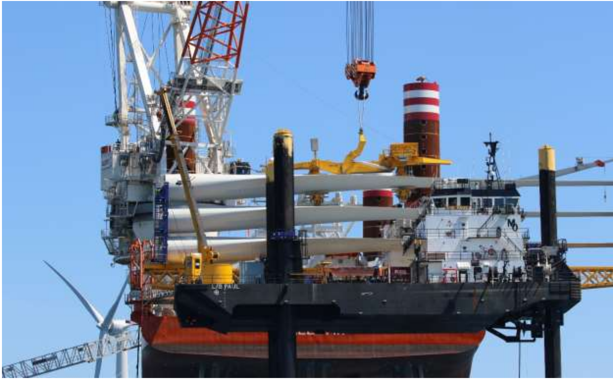
Figure 18. L/B Brave Tern lifting turbine blades from L/B Paul.
